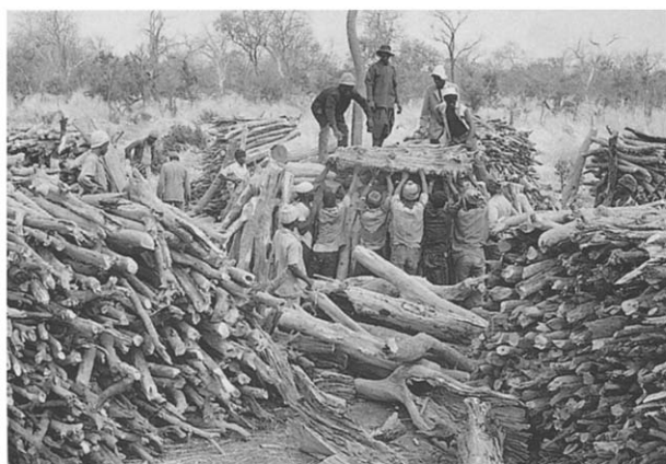
Figure 5. Kilé Ranso – a kiln building work party. Surga are helping each other in building the core of a kiln.
