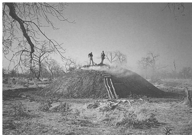
Figure 6. Surga tending the firing of a kiln. The kiln must be monitored round the clock for the one to three weeks it takes to carbonize the wood.
